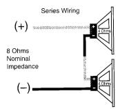
When the GTS180 is in bridged mode, the combined impedance of the speaker (or speakers) connected to the bridged channel should be at least 4 ohms. Sustained operation of the GTS180 in bridged mode with less than 4 ohms will likely cause overheating. If monaural operation is desired, and two 4-ohm speakers are used, it is best to connect each speaker to an individual amplifier channel and use the "L+R" mode on the input-mode switch to provide monaural operation.
