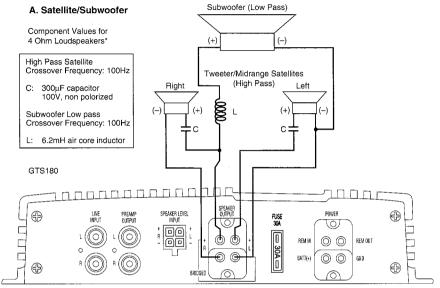
\*You may change the subwoofer satellite crossover frequency by using the Inductor and Capacitor values calculated with the following formulas:
